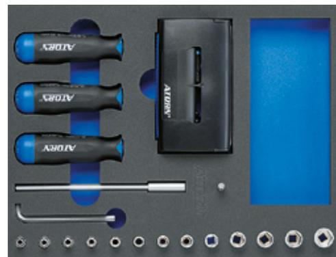
**Scope of delivery:** 1 ATORN torque screwdriver each 0.6 to 1.5 Nm, 1.5 to 3.0 Nm, 3.0 to 5.4 Nm, 1 ATORN socket wrench each 1/4" 4.0/4.5/5.0/5.5/6.0/7.0/8.0/9.0/10.0/11.0/12.0/13.0/14.0, ATORN bit holder for blades 170 mm, 1/4" bit holder, ATORN bit adapter for cordless drill 1/4", ATORN Bit box Collector Universal 61 pieces
