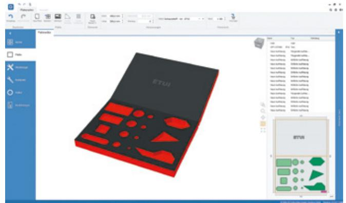
The quick and easy configurator for your individual hard foam inserts. Hard foam inserts can be custom-made for tools from the current HAHN+KOLB-product range and tailored to your existing drawer dimensions. With just a few clicks you can plan and design completely individual hard foam inserts that are equipped with tools and adapted to your wishes and needs.
